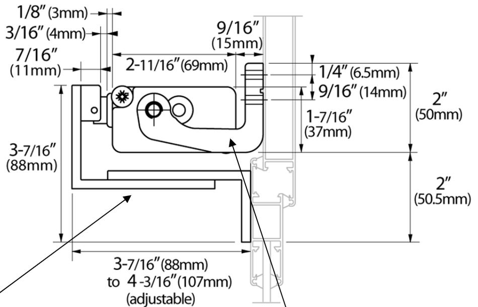
Adjustable Hopper Bracket (attached to sash)
