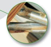
After just one year the red rust had spread from rivet joints on the surface of the arms and was bleeding and staining the surface of the PVC.
