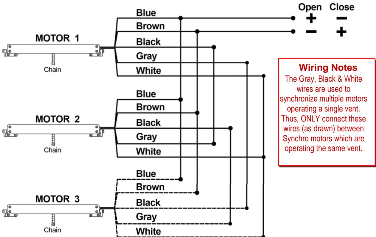
**Sample Wiring Diagram C: for connecting 4 DC Synchro-Quasar-L motors**
