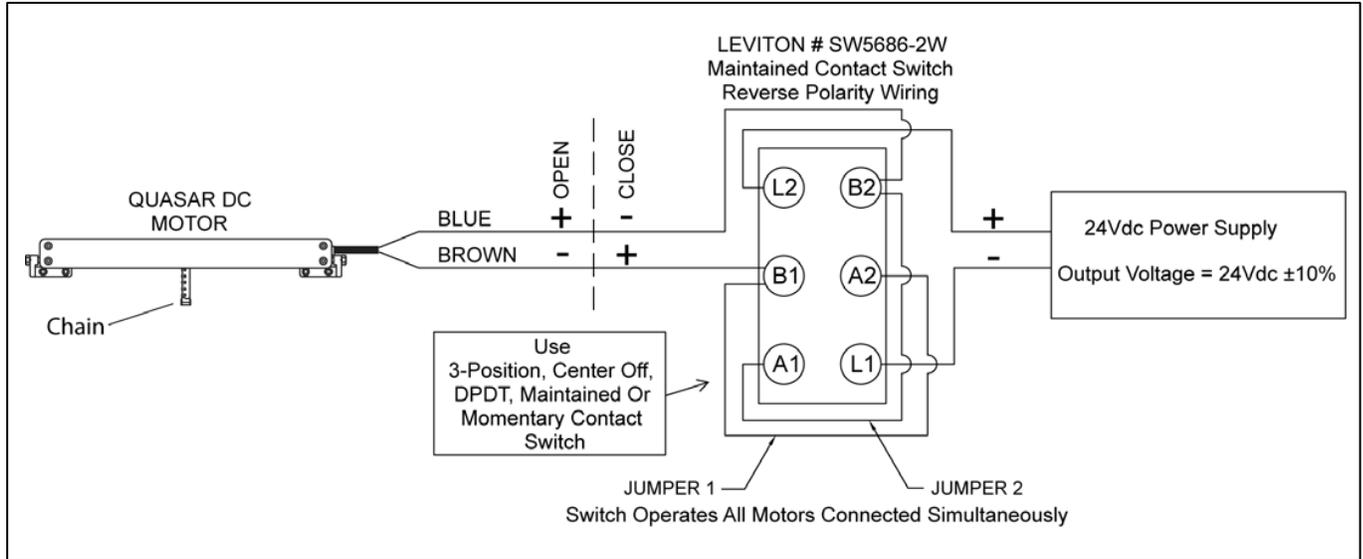
**Operation of Maintained Contact Switch DPDT (Double Pole-Double Throw):**
