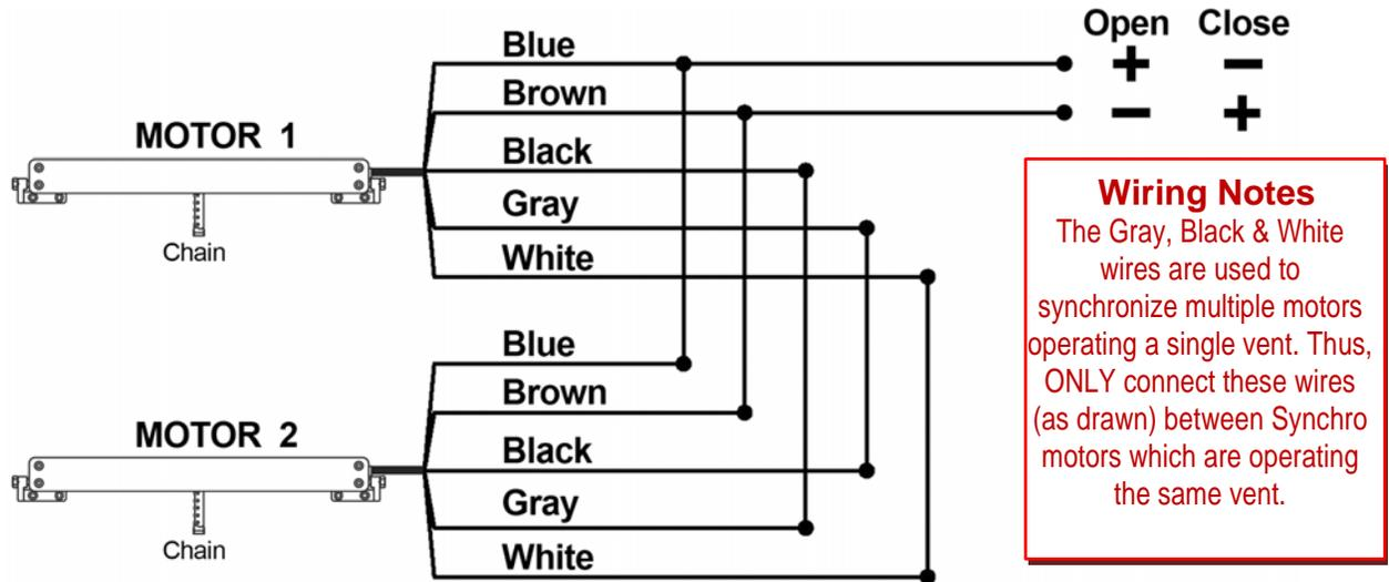
Sample Wiring Diagram B: for connecting 3 DC Synchro-Quasar-L motors
